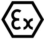
Drives that are suitable for use in explosion-prone areas comply with guideline 94/9 / EC (ATEX). Only drives that have the symbol on the side on the name plate may be used in explosion-prone areas. Notes in these operating instructions that must be observed are also marked with the explosion symbol.
